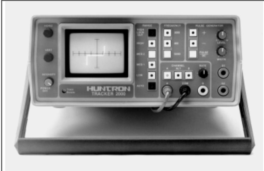
**Test components and boards without power - ideal for catastrophic failures**
