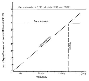
A comparison of different counting techniques shows the exceptional resolution achieved at all frequencies by the combined TEC and recipromatic techniques used in models 1991 and 1992. This outstanding resolution also applies to timing measurements which is not the case using other techniques.
