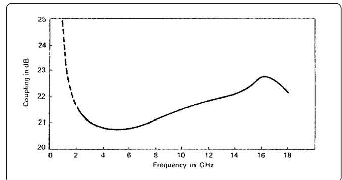
Figure 3. Typical coupling curve.
