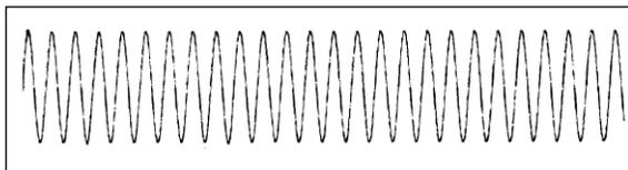
Figure 1. Basic 10 kHz sine wave:  $F1 = \text{SIN}(10K*t)$
