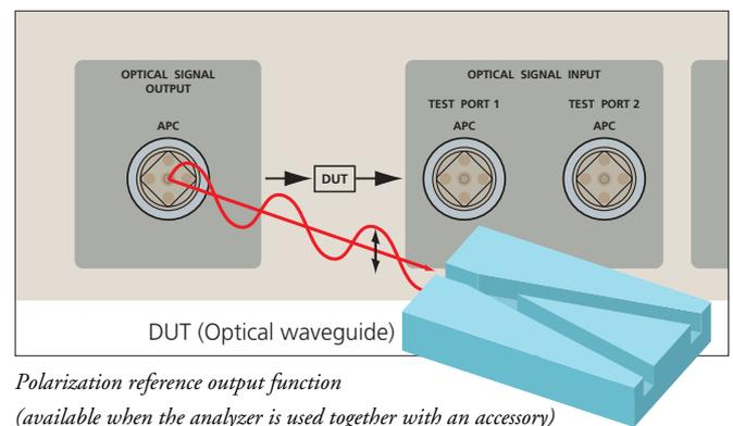
Polarization reference output function
