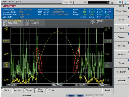
IL/PDL characteristics of AWG
